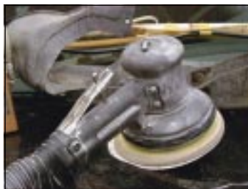
Orbital sander with integrated extraction for connection to a high vacuum installation.
