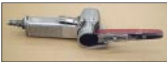
Belt sander. If these sanders are used – use tools with integrated extraction or hold the hose from a high vacuum installation beside the tool
